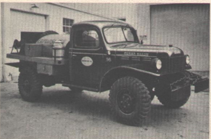
"Explosive" truck is always part of the seismic exploration fleet. Ability to move right up to location eliminates rehandling of explosives.
