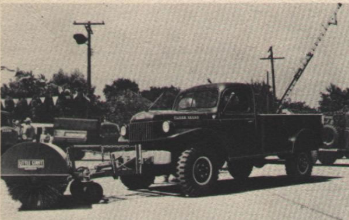
Street sweeping. Rotary sweepers are conveniently installed on the front of the POWER-WAGON.
