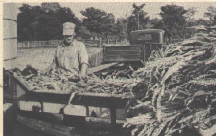
Ensilage cutting equipment . . . in fact, various types of farm machinery can be driven from the POWER-WAGON power take-off.
