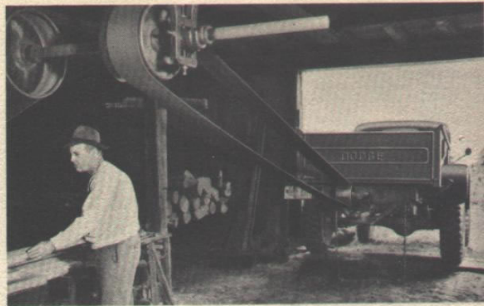
Buzz saws and saw mill equipment are operated with belt from pulley, mounted on tail shaft of the POWER-WAGON.
