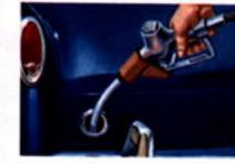
STERN SIDE FUEL FILLER is very convenient. Located at the rear of car, station attendant can reach it with hose from either side. No need to drag hose over rear deck when filling.
