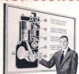
Dodge "Job-Rated" trucks offer a high compression ratio of 7.0 to 1 on models through 1-ton. This results in top efficiency with flashing power. Here's real economy with outstanding performance—to give you more power from every drop of fuel.
