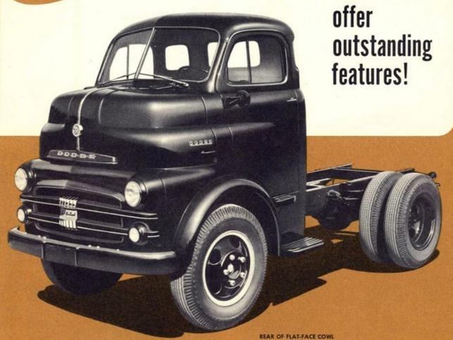
Dodge "GM" and "HM" cab-over-engine models are more compact than conventional cab models... and thus require a much shorter wheelbase to accommodate the right C. A. dimension for a given body length. In fact, with a C.O.E. model you can use a much longer body than would be possible on a conventional cab model of a comparable wheelbase.
