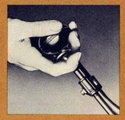
This convenient button on the gearshift lever operates the vacuum-actuated power shift. The driver can shift the axle alone or he can "split shift" so that both axle and transmission ratios are changed at the same time.
