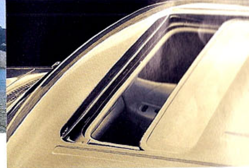
Available power moonroof with the one-touch-open feature can be tilted up or opened completely.
