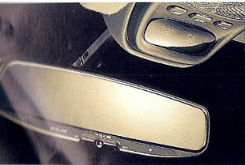
Electrochromic rearview mirror detects high/low beams and adjusts automatically for excellent visibility.
