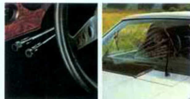
Stalk-mounted controls on steering column (L) Oscillating Fluidic Windshield Washer System (R)
