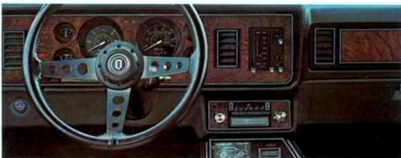
Capri's full instrumentation includes tachometer and oil pressure, temperature and ammeter gauges
